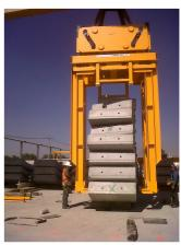
An embedded hydraulic power station allows a power supply to the opening and closing jacks by radio control. On the building site in Hong Kong the clamp is **equipped with an approved control device with double transmitter**, in order to have one on the surface and a second inside the access shaft without risking interconnections between the transmitters. A battery rack, easy to disassemble from the clamp, ensures the power supply of the system.
